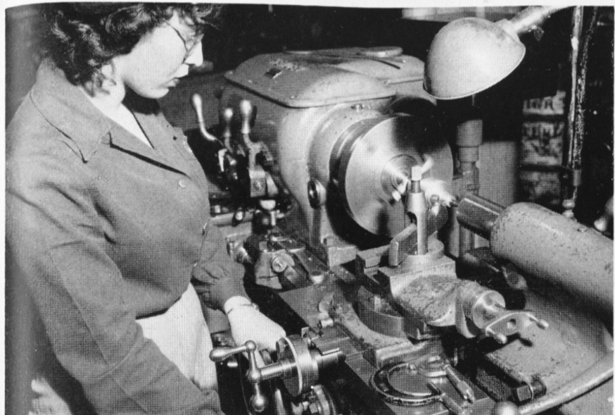
Here is Margaret Iorio at the lathe in the process of turning a draw punch for use in the Redraw Department. She started with a bar stock. She will complete the machining of the work to the point where the job will be ready for the Hardening Room.
