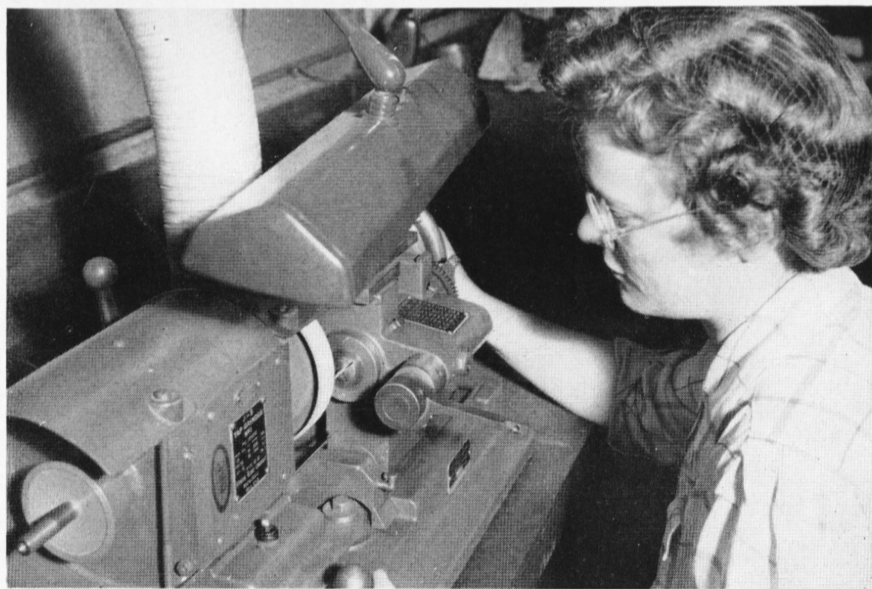
Alice Nolan, at the tap grinder, makes cutters to mill the powder grooves of fuses. She first grinds for diameter; then for clearance. Good eyesight and meticulous attention to the work are necessary here. She and her co-workers have demonstrated their ability for this work.
