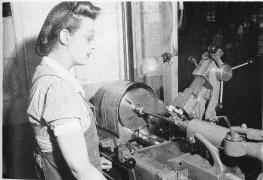
Helen Medhurst, who has become an experienced and skillful worker, is operating a superfinishing machine on the final surfaces of a tapered plug for the Tube Mill. This is an exacting job. Helen does it well. With skill and care she is supporting the servicemen.
