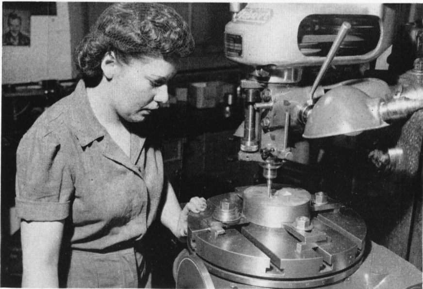
Jeannette Forest is considered by her superiors an excellent all-around mechanic. She is milling a die for the Forge Room. She does all the complicated calculations required to sink cavities in the side of the punch.
